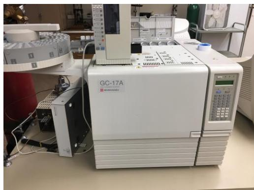
The Shimadzu GC-17A is designed to separate the different compounds in a mixture and is specifically helpful in determining the fatty acid content of many meat and dairy products.
