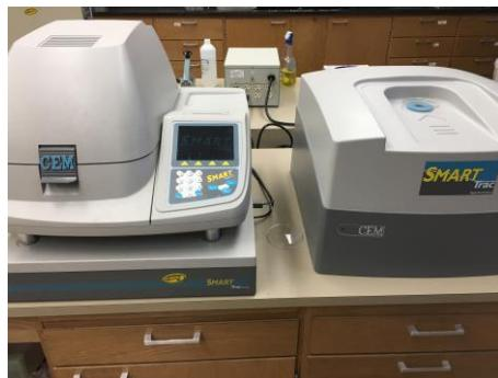
In raw and processed meats, milk, and other biological mixtures the CEM Smart System 5 with Smart Trac Rapid Fat Analysis can be used to determine the total moisture and fat in an accurate and timely manner using microwave and nuclear magnetic resonance (NMR) technology.
