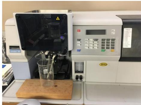
The AAnalyst 100 is an atomic absorption spectrometer that uses flame absorption and flame emission techniques to measure the concentration of over 70 different elements in liquid or solid samples.
