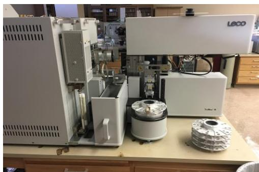
The Leco TruMacN uses nitrogen determination to give accurate and precise protein determination for feeds, grains, seeds, meat products, milk, urine, fecal products, and many other biological samples.
