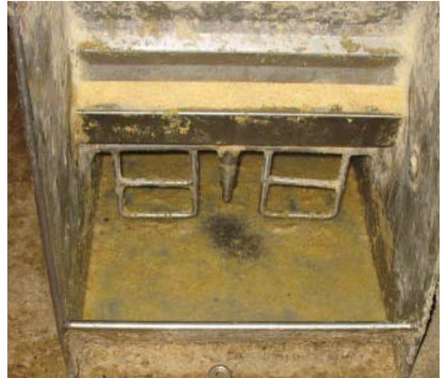
Setting of 14 with a 1 inch opening and ~73% coverage
