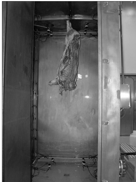
ESS cabinet dimensions were 6 feet × 5.87 feet × 11.42 feet.
