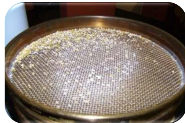
Step #4 Record Weight on Sieve
