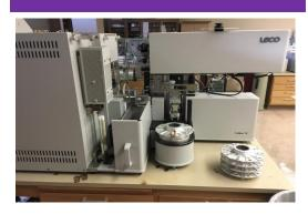
The Leco TruMacN uses nitrogen determination to give accurate and precise protein determination for feeds, grains, seeds, meat products, milk, urine, fecal products, and many other biological samples.
