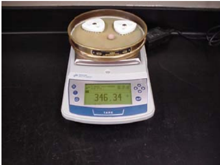
Step 2: Weigh each empty sieve along with its ball and carnucle(s).
