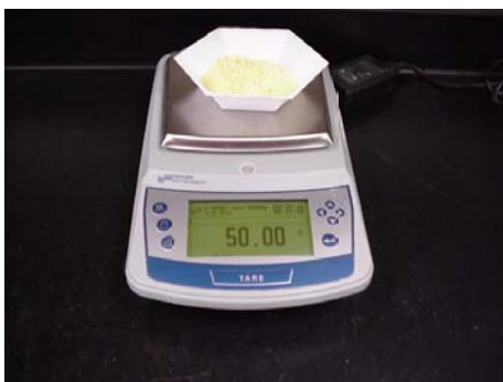
Step 4: Weigh 50g of sample & pour into stack, placing lid on top.
