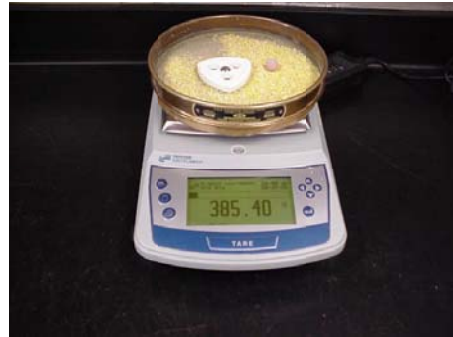
Step 6: Weigh each sieve with its ball, carnucle(s), and sample collected.
