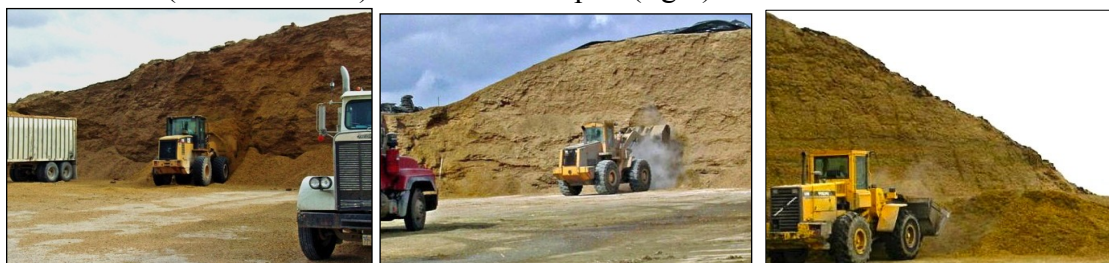
Figure 2. The payloader operators are at risk from collapsing corn silage in the over-filled bunker silos (left and center) and over-filled pile (right).
