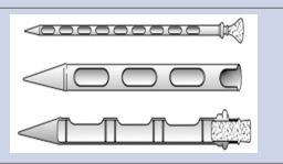
**Figure 2:** Manual slotted grain probe. Reproduced with permission from Herrman.<sup>3</sup>
