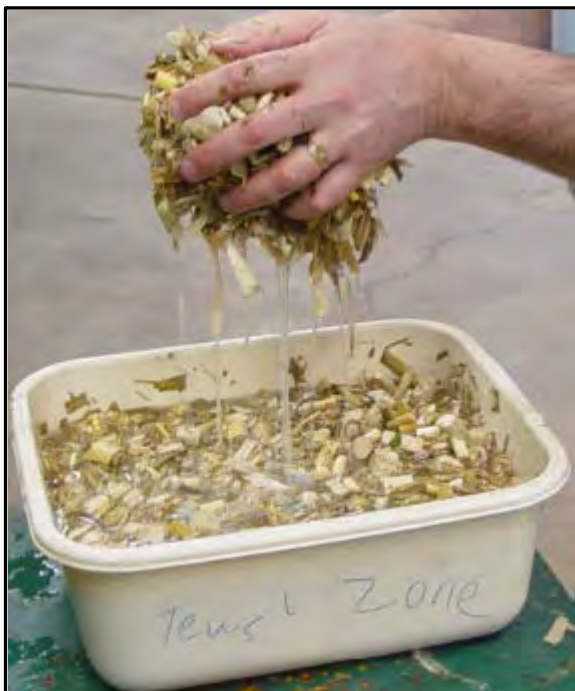
Figure 3. Skimming and removing the floating stover.
