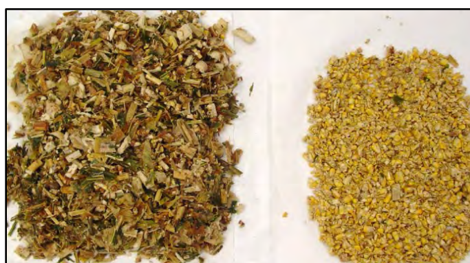
Figure 5. Example of separated stover and kernel fractions using the water separation technique.
