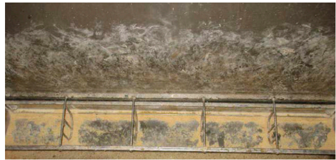
Figure 7. Conventional dry feeder with a 2.03- to 2.72-cm opening (Setting 8) and approximately 21% trough coverage. See online version for figure in color.
