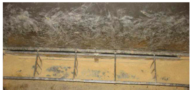
Figure 8. Conventional dry feeder with a 2.76- to 3.44-cm opening (Setting 10) and approximately 79% trough coverage. See online version for figure in color.
