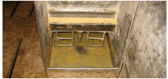
Figure 4. Wet-dry feeder with a 1.91-cm opening (Setting 10) and approximately 57% trough coverage. See online version for figure in color.
