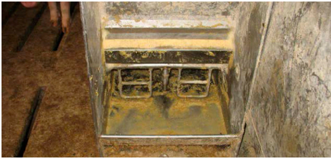
Figure 3. Wet-dry feeder with a 1.27-cm opening (Setting 6) and approximately 35% trough coverage. See online version for figure in color.
