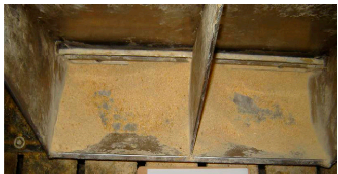
Figure 5. Wide feeder adjustment (minimum feeder gap opening was 2.54 cm with a maximum gap of 3.81 cm) averaged 83% feeder pan coverage, Exp. 2. See online version for figure in color.
