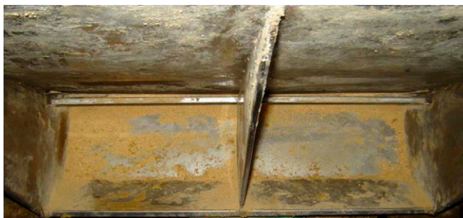
Figure 1. Narrow feeder adjustment (minimum feeder gap opening was 1.27 cm with a maximum gap of 1.91 cm) averaged 27% feeder pan coverage, Exp. 1. See online version for figure in color.
