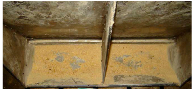
Figure 3. Wide feeder adjustment (minimum feeder gap opening was 2.54 cm with a maximum gap of 3.81 cm) averaged 75% feeder pan coverage, Exp. 1. See online version for figure in color.
