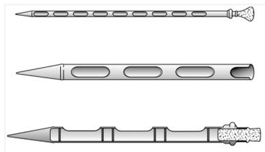
**Figure 1.** Slotted grain probe (Herrman, 2001)
